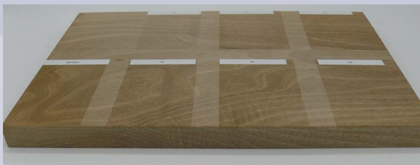
Fig.1 First application tests of the wax emulsions for the care of oak surfaces in direct comparison to conventional formulations containing carnauba wax. © hollu Systemhygiene GmbH (Research & Development Department)
