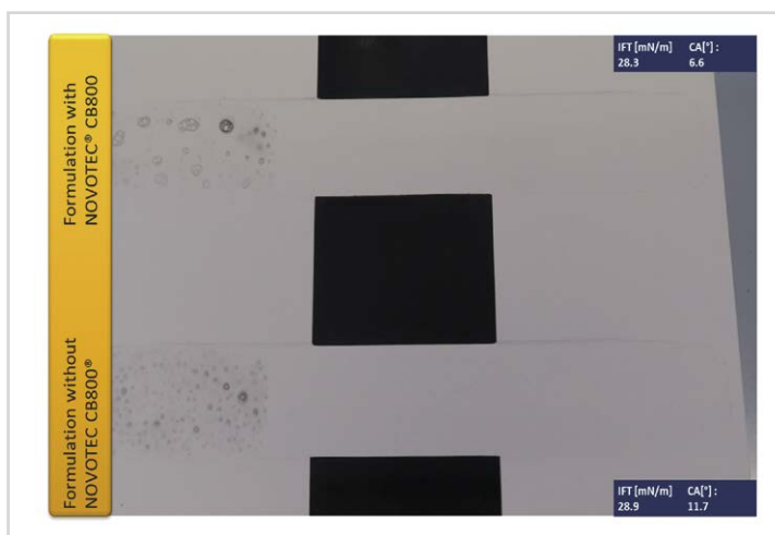
Fig. 4 A tile pre-washed with concentrated cleaner with/without NOVOTEC® CB800 and cleaned again with the respective cleaners shows only a minor improvement due to protein protection of the first cleaning.
