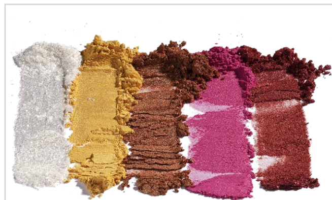
Fig. 2 The shiny effect of pearlescent pigments results from the platy structure that reflects the light like a mirror.
