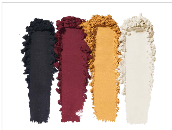
Fig. 3 Appearance of the 4 different color pigments of the Ronastar® Allure series with 2-in-1 performance. (INCI: Black: CI77499 (Iron Oxides), Silica, CI 77891 (Titanium Dioxide), Mica; Red: CI77491 (Iron Oxides), CI 77891 (Titanium Dioxide), Silica, Mica; Yellow: CI 77492 (Iron Oxides), Mica, Silica; White: CI 77891 (Titanium Dioxide), Mica, Silica, Tin Oxide).
