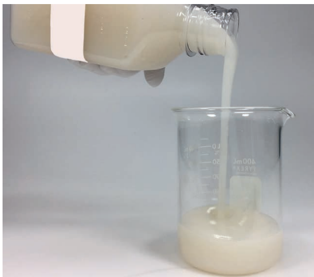
Fig. 1 Fermentation-Derived Cellulose comes ready to use and does not require pH adjustment or high shear mixing to be functional. Use levels range from 0.5% to 5% depending on the formulation and what is to be stabilized.
