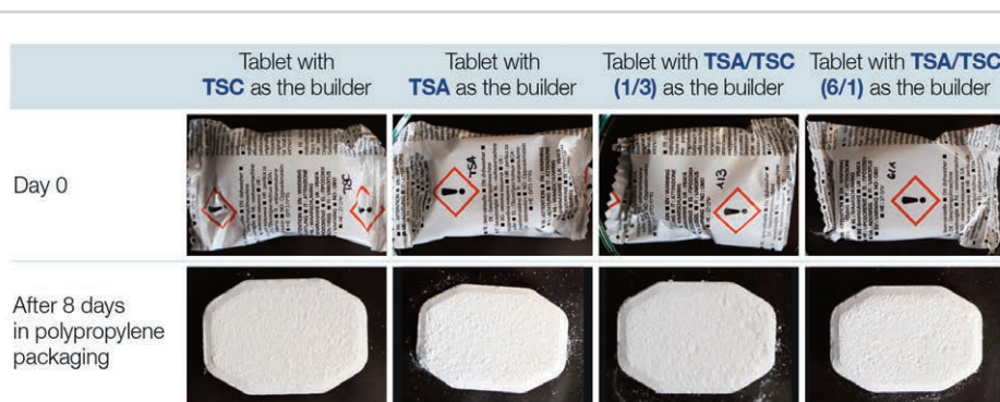
Fig. 4 The choice of TSA, TSC or mixtures thereof as builders has no impact on storage stability in polypropylene packaging.
