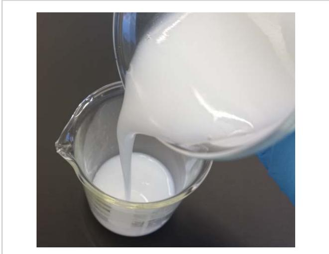
Fig.1 A representative picture of the homogeneous texture and pouring behaviour of formulations containing Exilva® cellulose fibrils at 0.5% w/w and cationic surfactant at 5% w/w.
