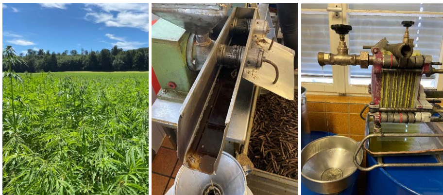
Fig.1 Left: Hemp field in Upper Swabia. Middle: Pressing of hemp seed oil using a screw press. Right: Filtration of the hemp seed oil.
