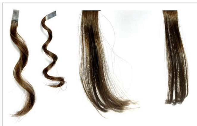
Fig. 6 The left side shows the improved curl retention properties and on the right side the reduction of static charge with WorléeStyle Eco 300/10-L3 , an ethanol-containing shellac solution compared to the placebo.
