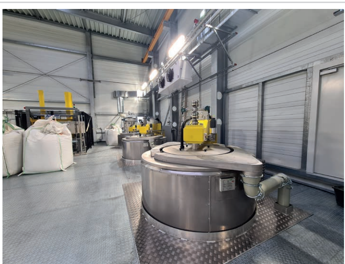
Fig. 3 Industrial CO 2 extraction plant for hops; source: Hopfenveredelung St. Johann GmbH
